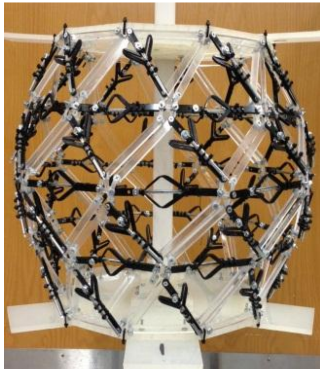
Figure 4.17 The spherical SMSF after applying vertical loading.
