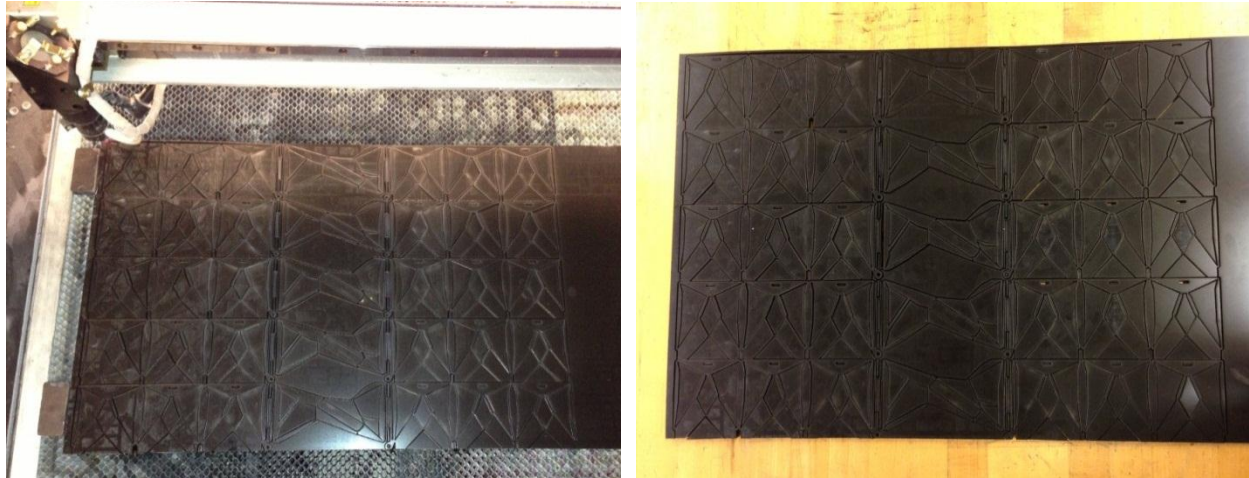
Figure 5.31 Laser cutting the mechanisms from Polypropylene Copolymer sheets.
