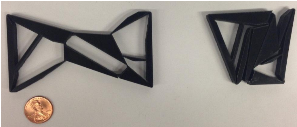
Figure 5.25 P_1 mechanism cut from Polypropylene Copolymer sheet.
